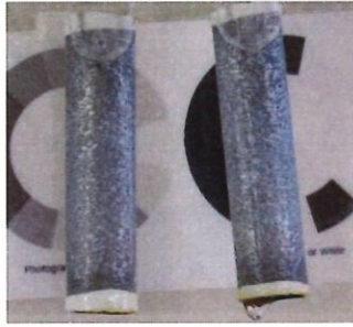
Photo 3: Electrical Conduit, Day 244, Fresh Water
