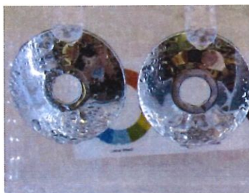
Photo 14: Escutcheon plate, Day 14, Fresh water.
