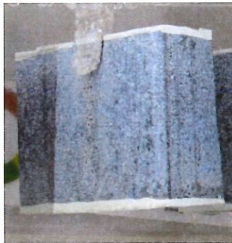
Photo 10: Sill plate, Day 244 Salt Water
