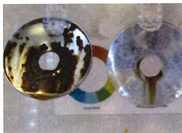
Photo 16: Escutcheon plate, Day 122, Salt Water
