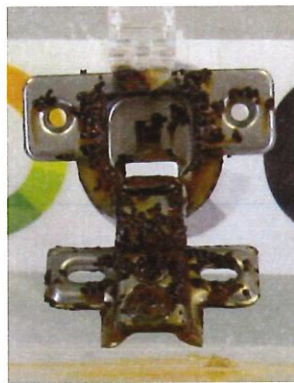
Photo 18: Concealed cabinet hinge, Day 122, Fresh water
