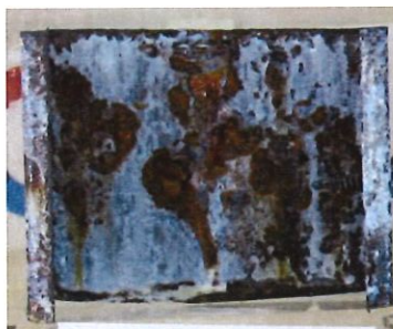
Photo 13: Framing, Day 461, Salt Water.
