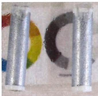
Photo 2: Electrical Conduit, Day 14, Fresh Water
