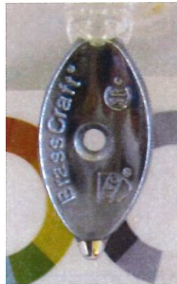
Photo 25: Angle stop valve, Day 122, Fresh Water
