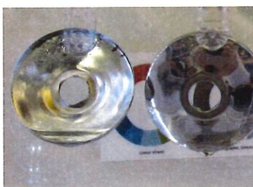
Photo 15: Escutcheon plate, Day 122 Fresh water
