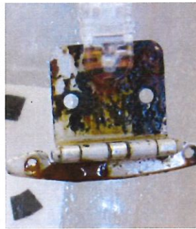
Photo 23 Face-mounted cabinet hinge, Day 122, Saltwater
