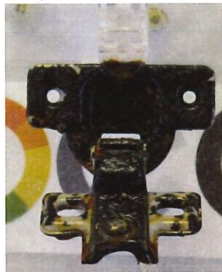
Photo 19: Concealed cabinet hinge, Day 122, Salt water
